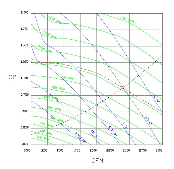
2400 CFM, 0.871 SP @ 1317 RPM and 1.455 BHP at 0 feet and 100 deg F  $\ast$  Please note that these curves were adjusted for job specific temperature and altitude.
